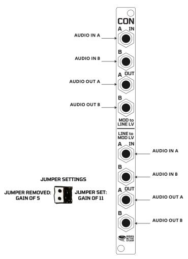
VERY LOW NOISE AND LOW DISTORTION CIRCUIT WHILE PRESERVING THE TRANSIENTS.
